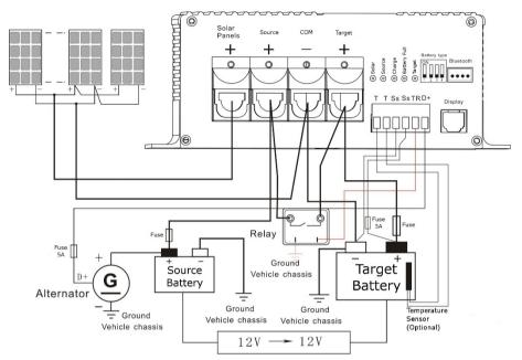
Connection diagram for DC1224-2530, DC2424-5030 & DC2412-6050:
